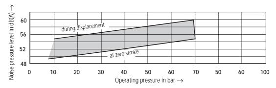
Measured in an anechoic chamber to DIN 45 635, sheet 26
