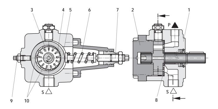
Hydraulic pumps of the type PV7...A are direct operated variable displacement vane pumps.
