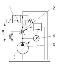
values) Operating pressure *p* →  $t_{\text{down}} / t_{\text{up}}$ 1 Directional valve (switching time 30 ms) 20 bar 2 Throttle for setting the pressure 3 Hydraulic pump  $t_{\text{down}}$ Time *t* – 4 Pressure test point  $q_{\text{V displacing}} \rightarrow q_{\text{V zero stroke}}$
