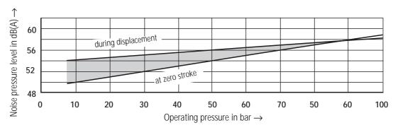
Measured in an anechoic chamber to DIN 45 635, sheet 26
