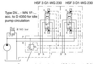
Pressure reducing valve type ADC 1-25 acc. to D 7458  $\,$
